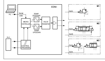
The EDM-M\* card is a digital amplifier for open loop proportional valves control by a PWM stage.
