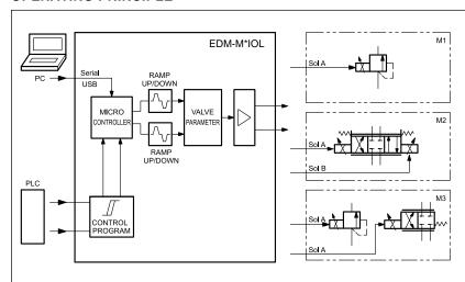
The EDM-M\*IOL card is a digital amplifier for open loop proportional valves control by a PWM stage.
