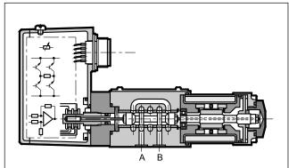
— The DXJ3 valve is a four-way servo-proportional valve where the spool moves inside a sleeve. This valve has a direct drive with a linear force motor resulting in high dynamic performances which are independent of system pressure. The spool position is controlled by a linear transducer (LVDT) with closed loop which
