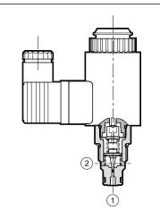
The PLKE08 valve is a proportional pressure control valve, direct operated, cartridge type. They can be used in blocks and manifolds with SAE-08 seat.
