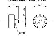
This indicator is a pressure gauge sensitive to the filter input pressure.
