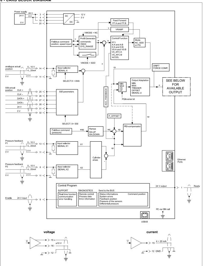
**NOTE**: If the card is configured as simple positioning control without pressure limitation then the output value is calculated just from the output of the position controller (CS) instead of apply MIN and MAX parameters. MIN/MAX are selected by the PQ\_INVERSE bit (Fieldbus).
