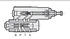
— MRQA is a pressure relief and safety valve with automatic unloading. Upon reaching the set value, the valve freely unloads the pump and puts it under pressure again when the pressure values descend in the circuit to correspond to 63% or 75% of the set value.
