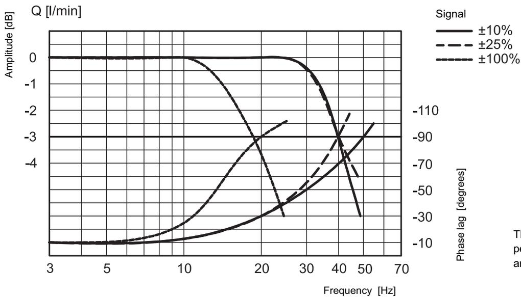
These test amplitude are performed with 50% of max flow, and  $\Delta p$  (P-T) 10 bar
