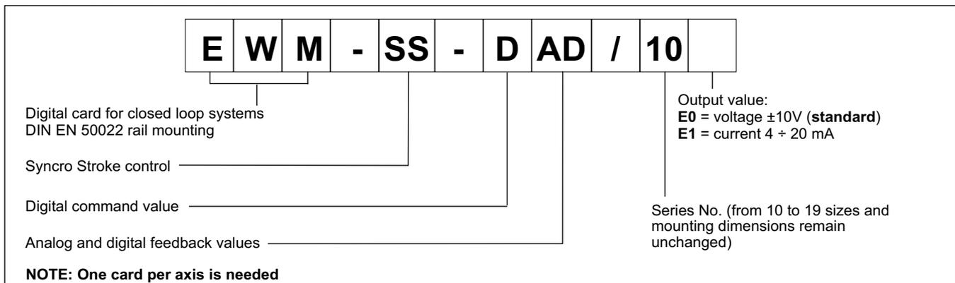
This electronic module is developed for controlling of hydraulic drives in synchronization. The communication with the PLC is solved by a standard Profibus DP interface. A typical repeatable positioning accuracy of up to 0,01% with analogue sensors or up to 0,001 mm with digital SSI sensors can be achieved. Proportional valves with integrated electronics (typically with control valves) can be driven by the analogue differential output.
